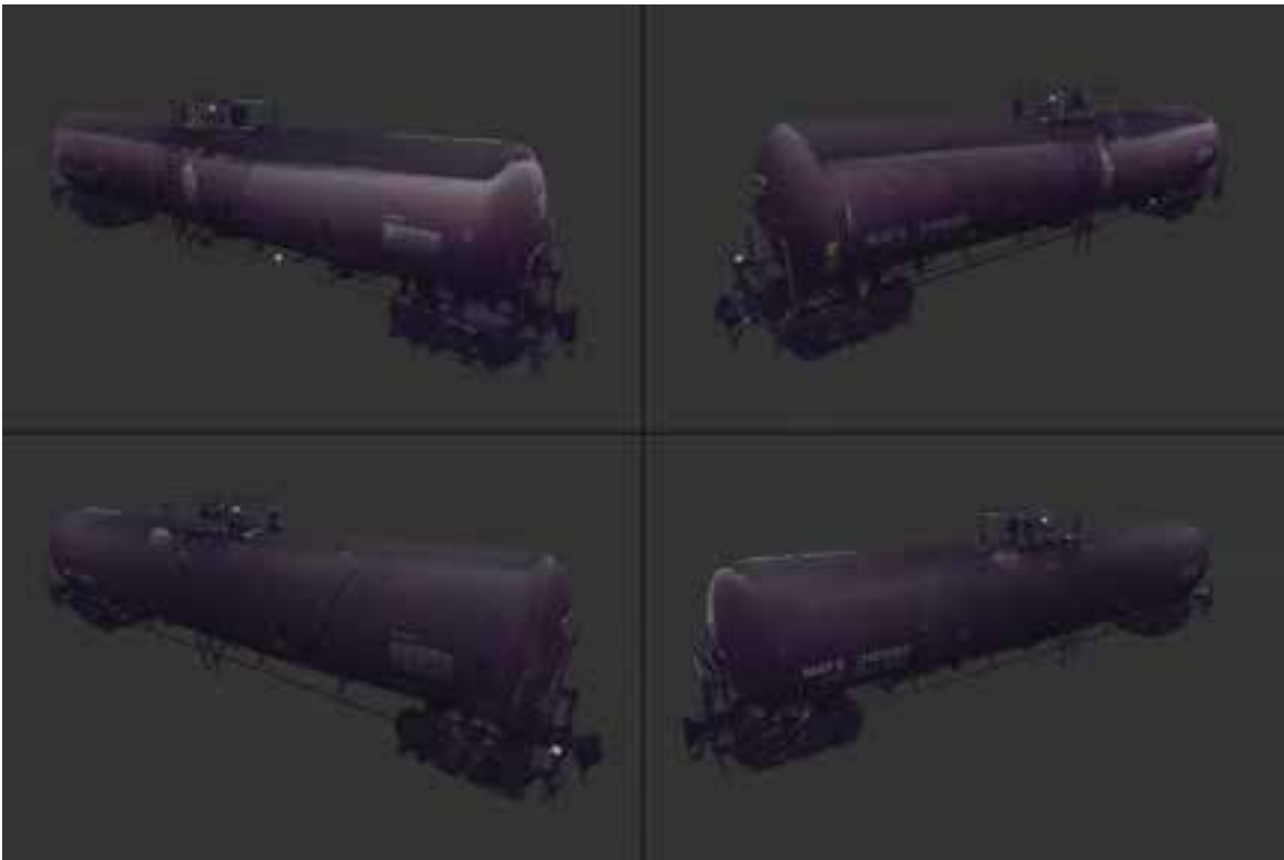
Figure 1: Oblique views of exemplar NATX 310595 tank car laser scan visualizations
