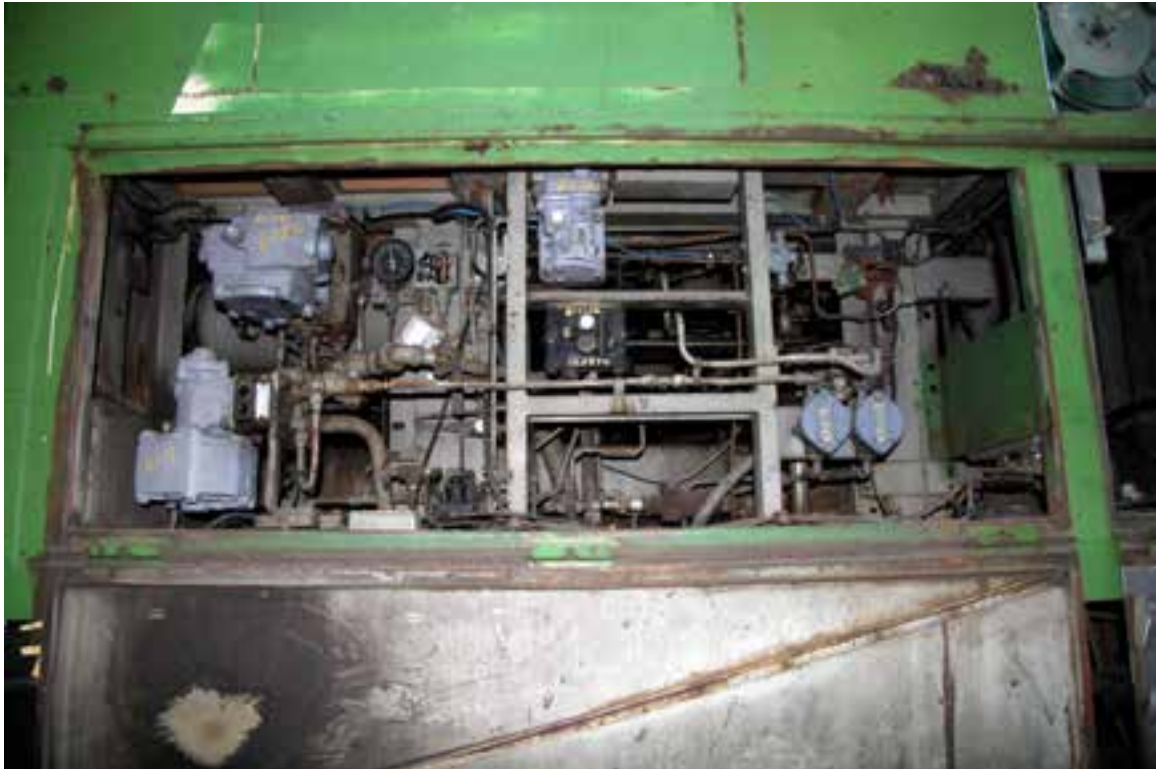
Figure 1: Locomotive 5017's airbrake compartment
