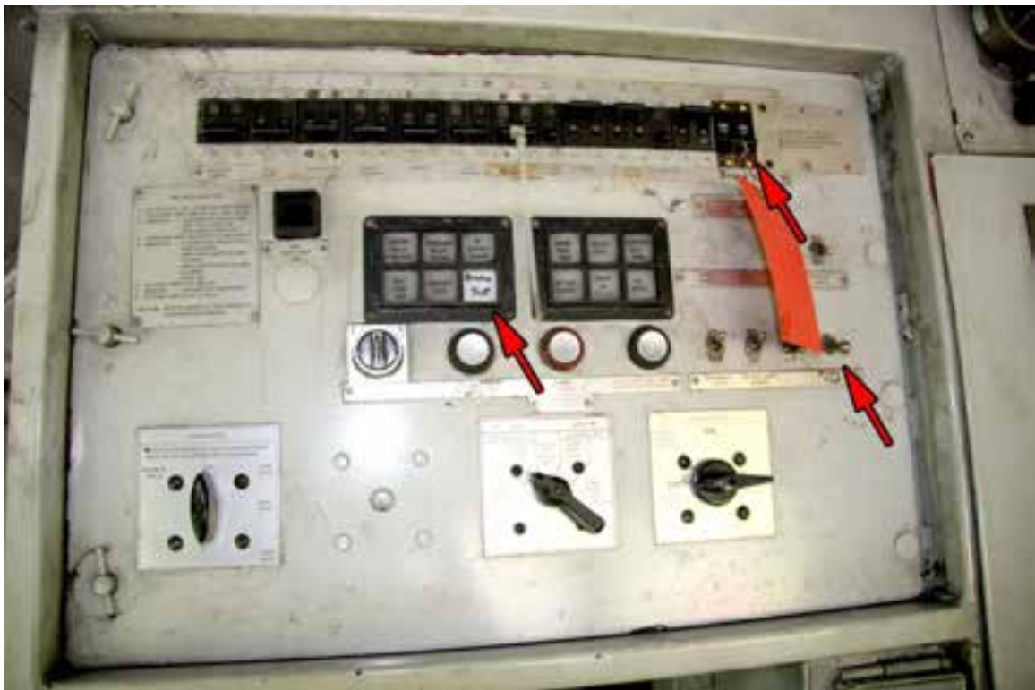
Figure 2: "Brake Test" components in locomotive cab
