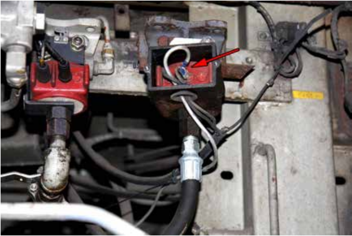
Figure 9: "Brake Test" connection for locomotive 5026
