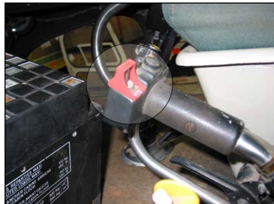
Photo 2. Hydraulic cut-off (HYD CUT OFF) switch
