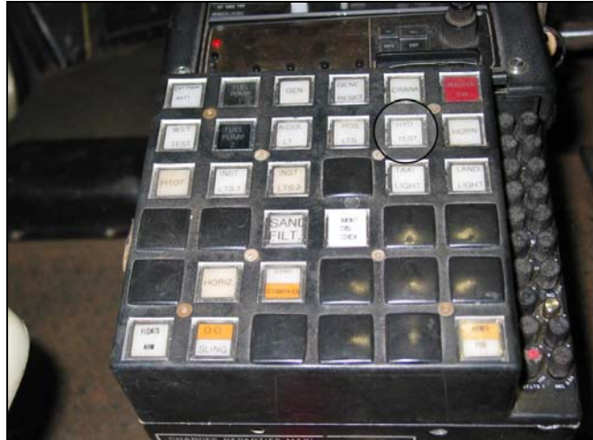
Photo 3. Hydraulic test (HYD TEST) switch
