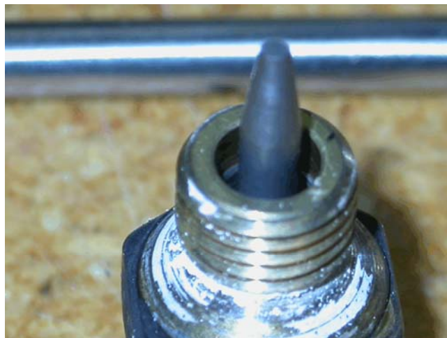
Photo 2. Fitting with excess thread sealant
