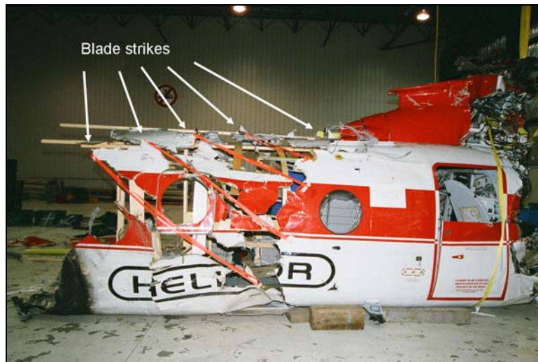
Photo 1. Fuselage blade strikes
