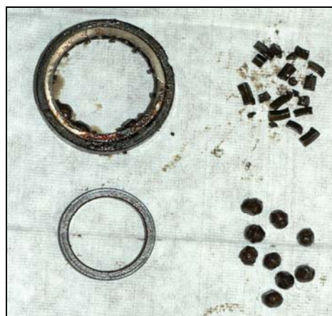
Photo 3. No. 3 bearing components disassembled
