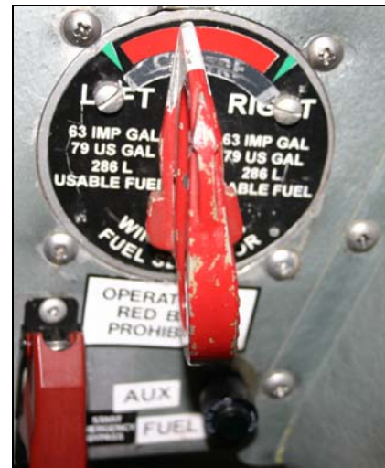
Photo 2. Wing tank selector
