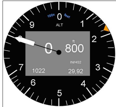
Figure 2. Pressure altimeter at 800 feet with the altimeter bug at 1180 feet
