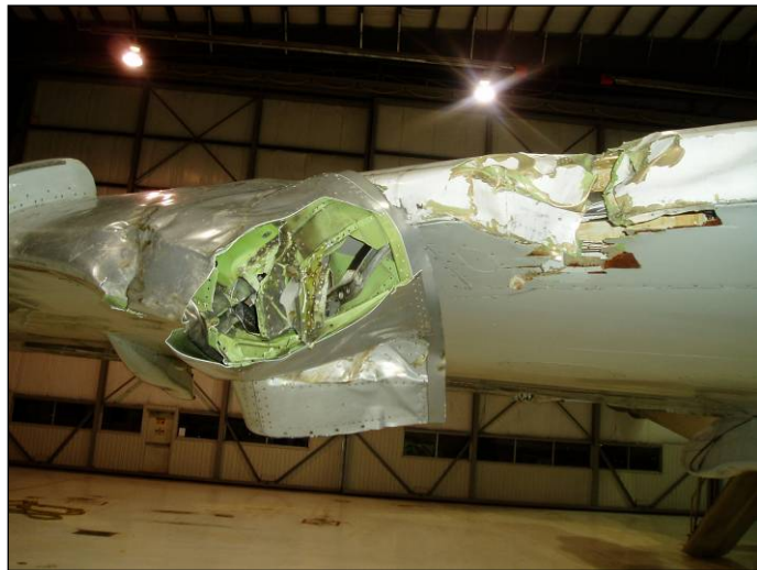
Photo 2. Aircraft damage – leading edge, right wing
