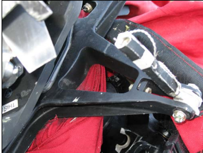
Photo 2. Doghouse cover wrapped between controls
