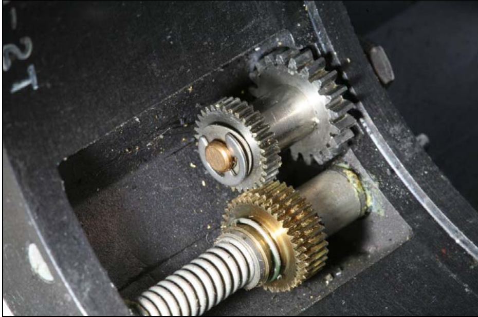
Barometric pressure/pointer setting gears
