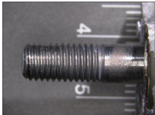
Photo 8. Top stud which remained in CHI91's MGB housing.
