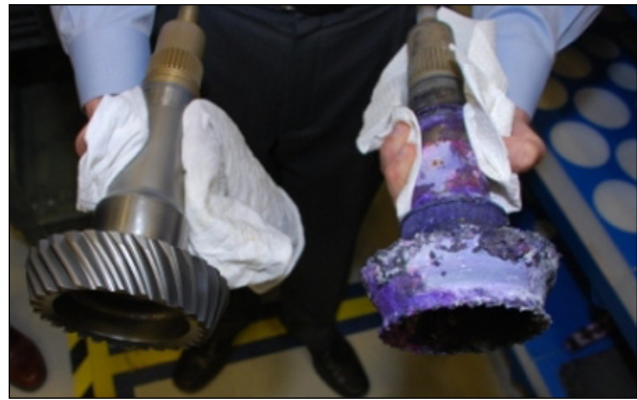
Photo 6. Damaged tail take-off pinion on right
