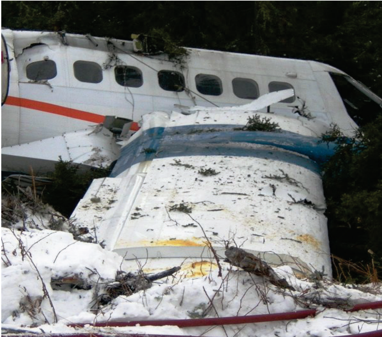
Photo 1. Right wing immediately after the accident
