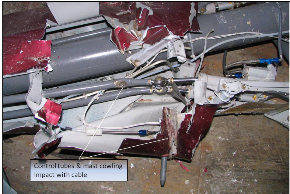
Photo 1. Cable marking on control tubes
