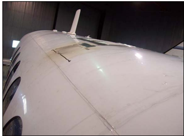
Photo 1. Damage as seen from outside aircraft
