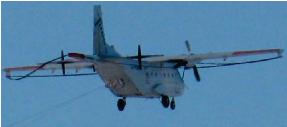
Photo 2. C-FDKM in flight with birds deployed. (Source: Jacqueline Thiessen, used with permission)
