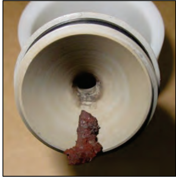
Photo 7. No. 2 ejector nozzle and foreign object debris
