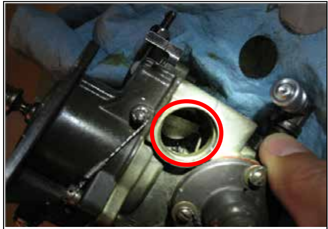
Photo 1. Bearing debris in PT governor (red circle)
