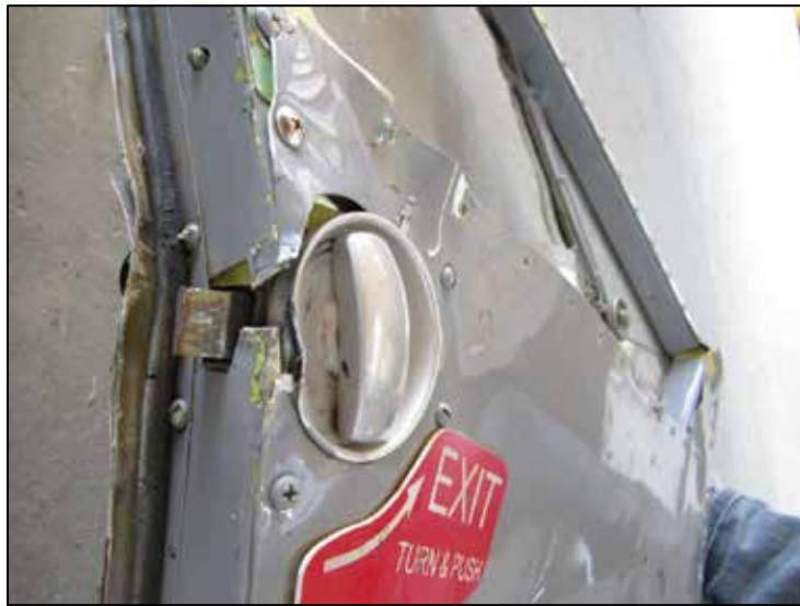
Photo 2. Pilot's door mechanism
