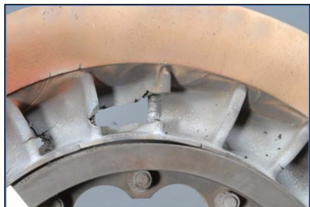
Photo 8. Stator vane burn-through
