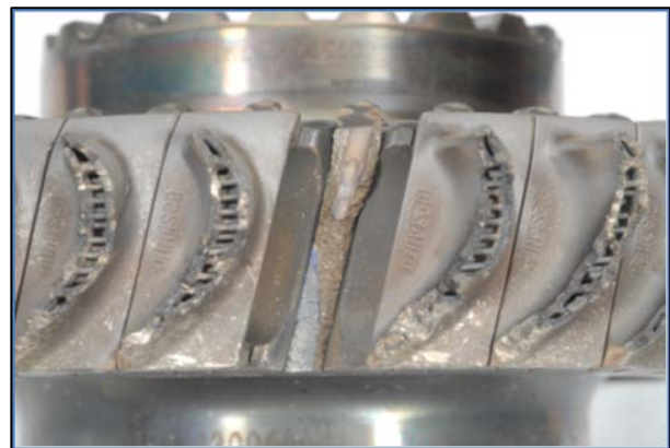
Photo 5. First-stage turbine wheel failure
