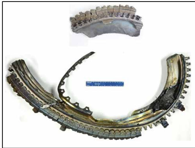
Photo 9. Recovered low-pressure turbine 1 segments (Source: Pratt & Whitney)
