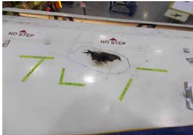
Photo 4. Left-wing upper surface damage showing burn marks (Source: Bombardier Inc.)
