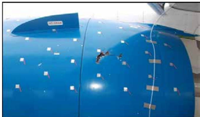
Photo 5. Damage to right-engine inboard thrust reverser cowl translating sleeve (Source: Bombardier Inc.)
