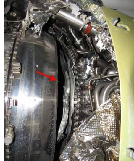
Photo 6. Example of a left-engine turbine case breach at the 3 o'clock position (Source: Bombardier Inc.)
