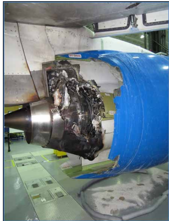
Photo 2. Left inboard thrust reverser cowl damage (Source: Bombardier Inc.)
