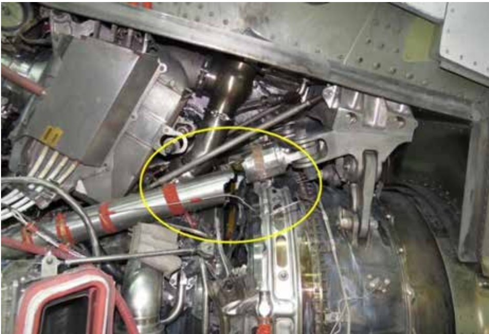
Photo 7. Damage to left-engine outboard thrust link and fire detection loops (Source: Bombardier Inc.)
