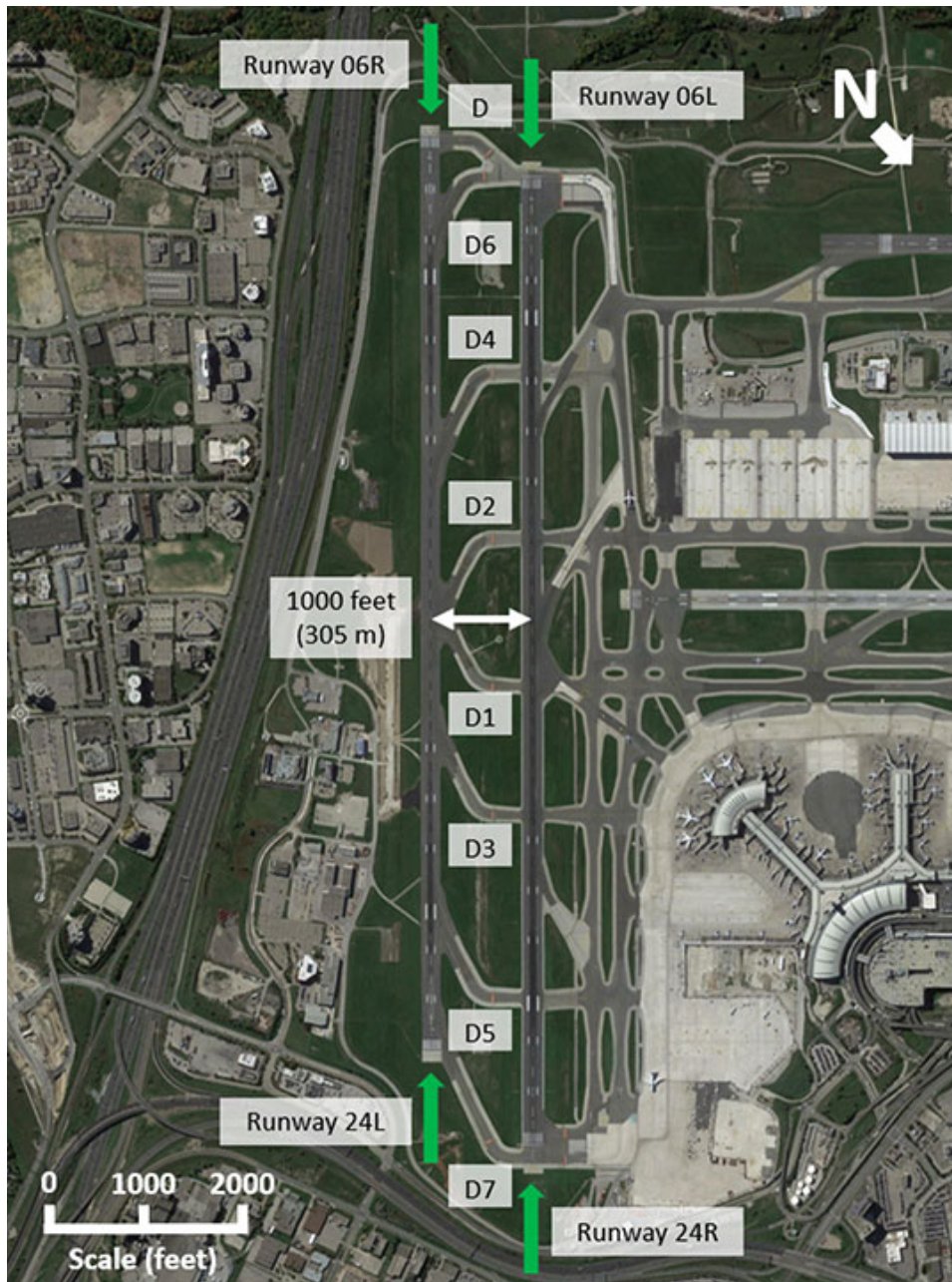
Figure 4. CYYZ's south complex runways and rapid exit taxiways (Source: Google Earth, with TSB annotations)
