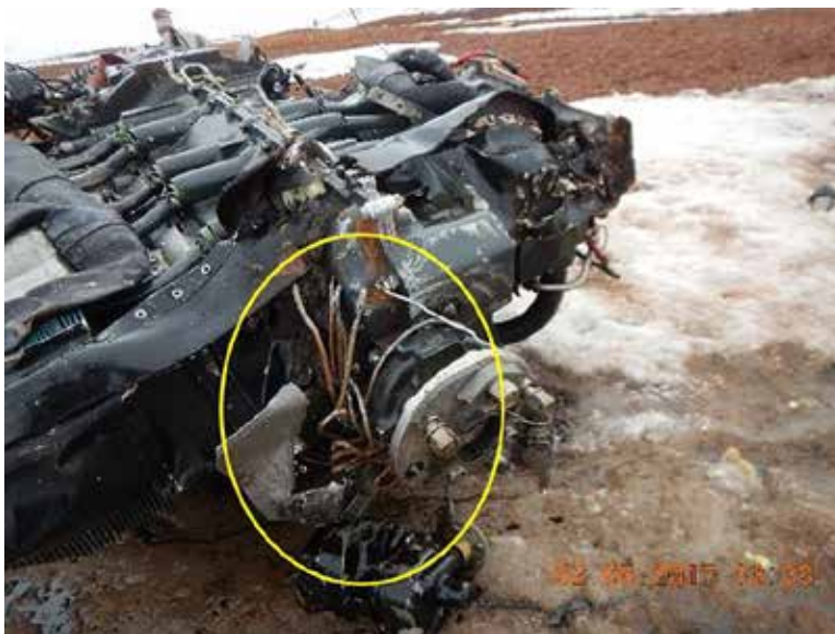
Figure 5. Left engine of C-FQQB: the circle shows the severed pieces of cable wrapped around the propeller drive shaft
