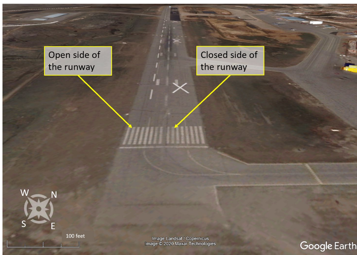
Figure 3. Aerial view of the runway markings used at the Iqaluit Airport during construction (Source: Google Earth, with TSB annotations)
