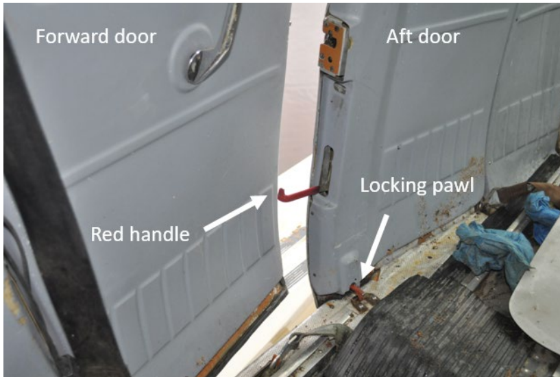
Figure 4. Rear double cargo door in the open position (Source: TSB, with annotations)
