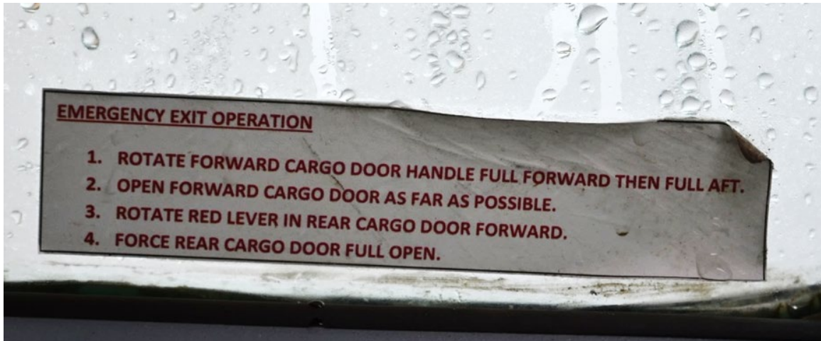
Figure 7. Instructions for operating rear double cargo doors as an emergency exit on the occurrence aircraft (Source: TSB)
