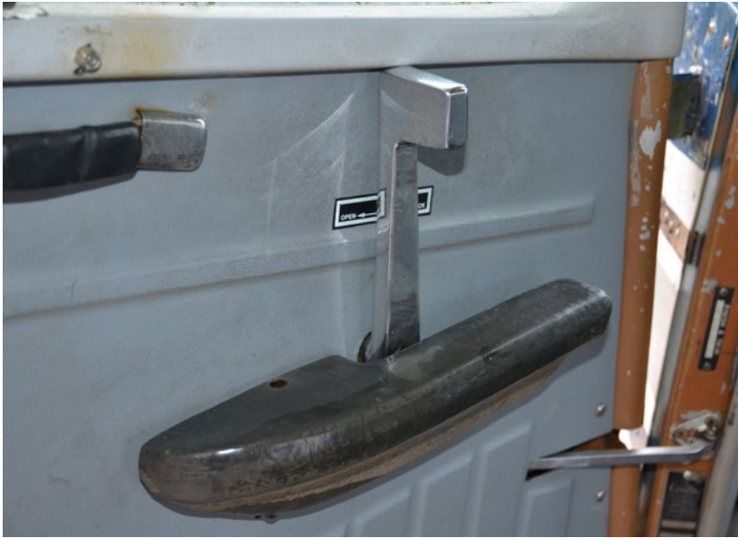
Figure 3. Pilot door handle in the closed position (Source: TSB)
