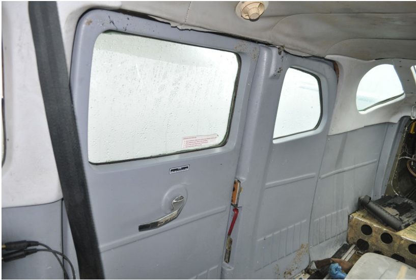
Figure 5. Interior view of the rear double cargo door in the closed position (Source: TSB)
