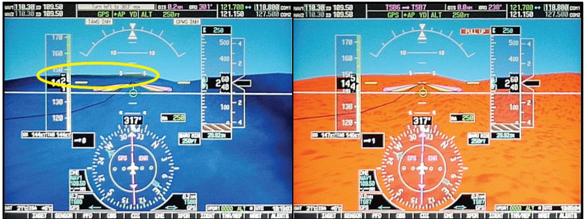
Figure 5. Comparison of the geometry of the surface textures depicting Addenbroke Island as shown on the aircraft's primary flight display with the forward looking terrain awareness inhibited (left image), and with the forward looking terrain awareness enabled (right image) when flown at 250 feet above ground level (Source: TSB)
