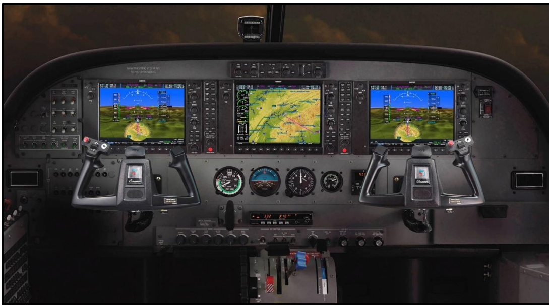
Figure 3. Garmin G1000 for the Cessna Caravan showing the primary flight display (left- and right-hand screens) and multifunction display (middle screen) (Source: Textron Aviation)
