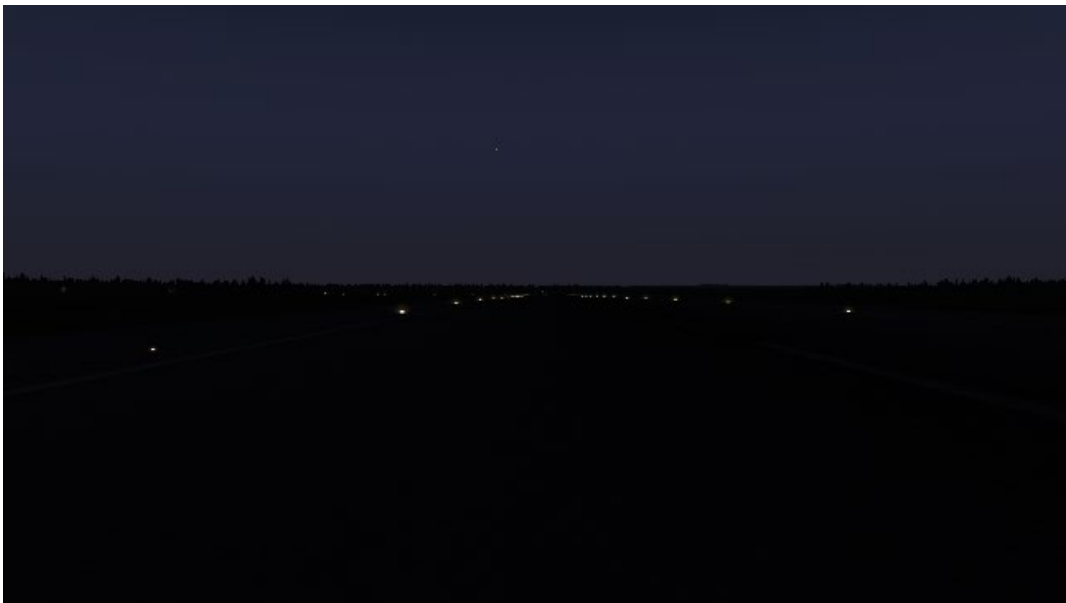
Figure 7. Runway edge lights seen by a pilot when the aircraft is 30 feet to the left of the runway centreline (Source: TSB, image created using the X-Plane Flight Simulator)
