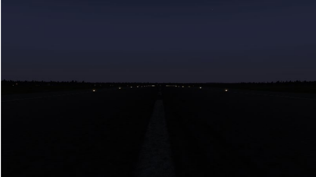
Figure 6. Runway edge lights seen by a pilot when the aircraft is on the runway centreline (Source: TSB, image created using the X-Plane Flight Simulator)
