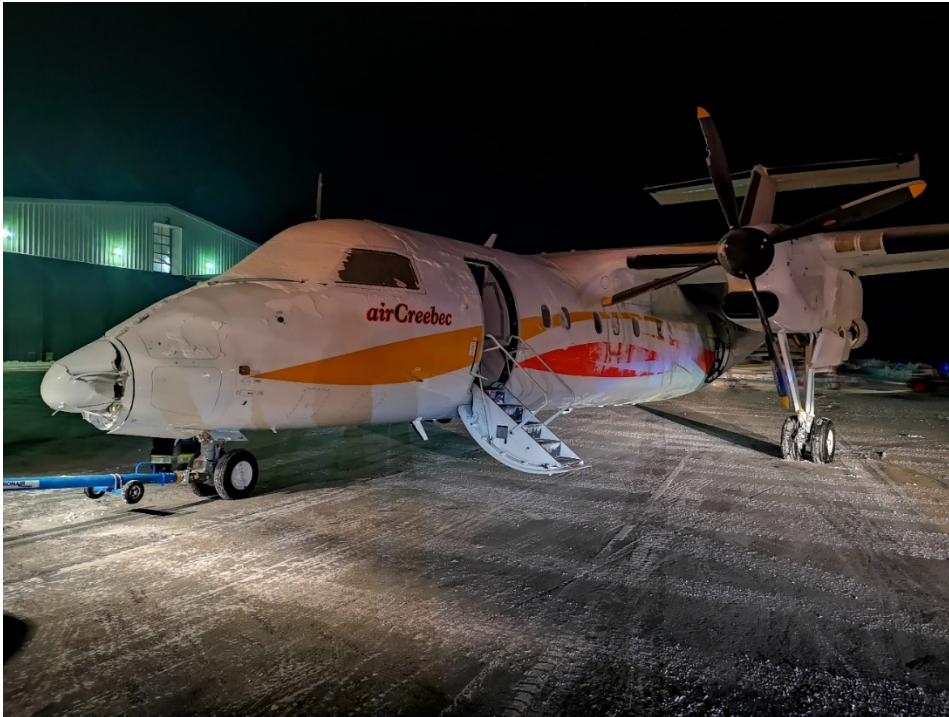
Figure 3. Aircraft after being towed; visible damage to the nose and propeller (Source: Air Creebec Inc.)
