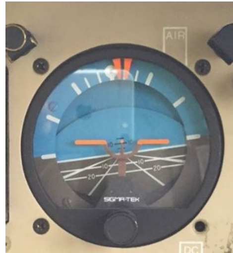
Figure 2. Right-side attitude indicator with no vacuum applied (Source: Air Tindi Ltd.)
