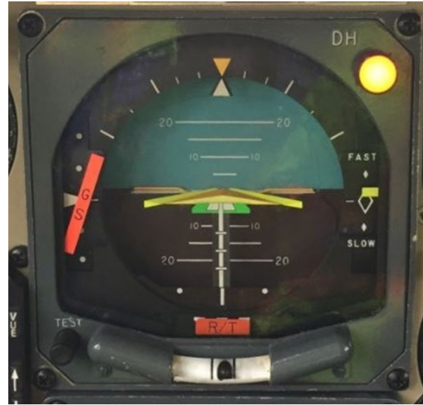
Figure 3. Left-side attitude indicator with power applied (Source: Air Tindi Ltd.)
