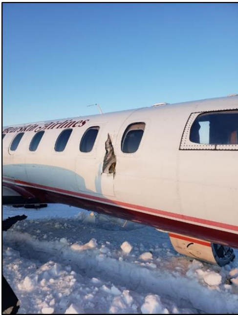
Figure 3. Right-side fuselage penetration (Source: Ontario Provincial Police)
