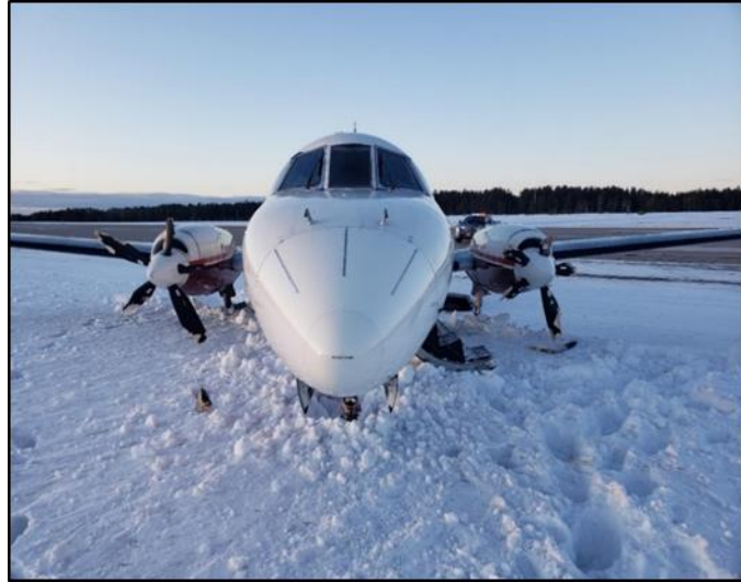
Figure 2. Shattered propellers (Source: Ontario Provincial Police)
