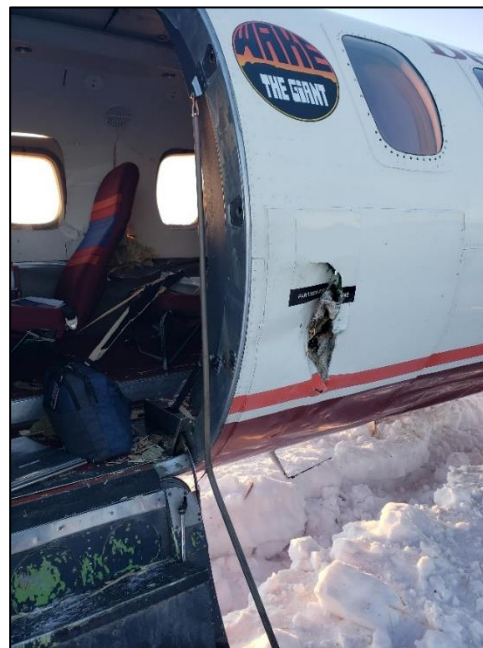
Figure 4. Left-side fuselage penetration (Source: Ontario Provincial Police)
