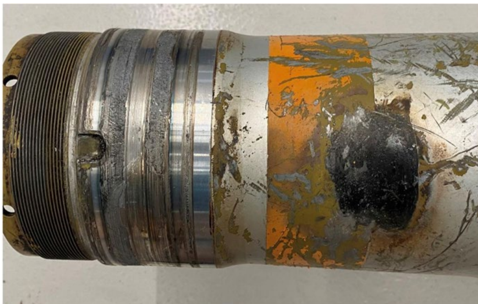
Figure 12. Friction marks on the No. 4 wheel axle damaged during the incident on 17 December (Source: Safran)
