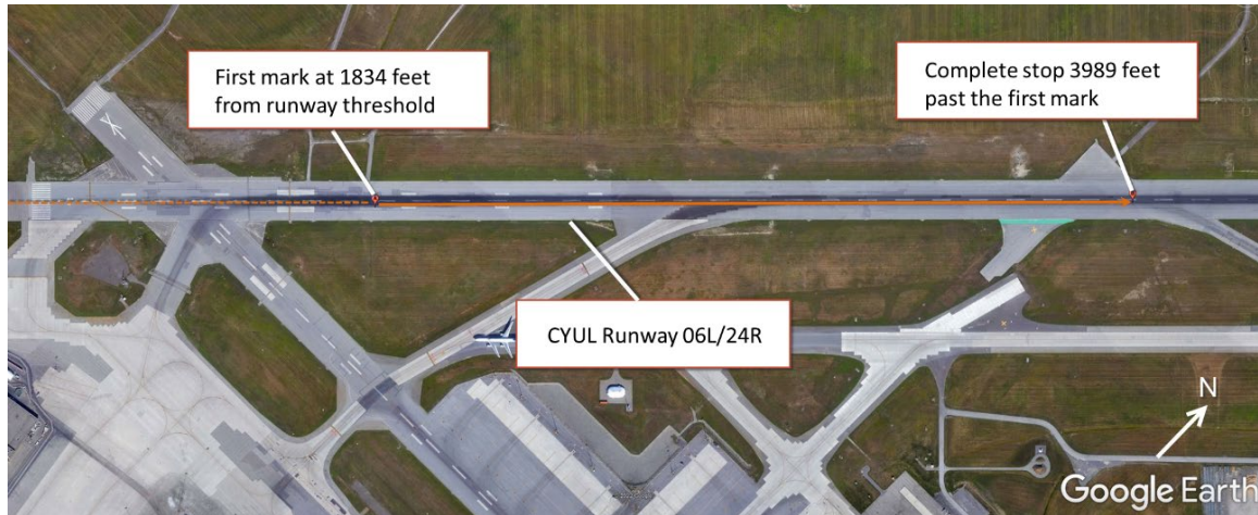
Figure 5. Aerial view of the relevant portion of Runway 06L indicating the distance travelled by the aircraft between the first damage mark and the stopping point (Source: Google Earth, with TSB annotations)
