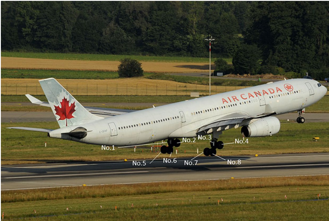
Figure 2. A330 main landing gears and wheel numbering (Source: Urs Ryser, with TSB annotations)
