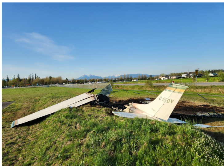
Figure 2. Occurrence aircraft wreckage after the post-impact fire (Source: TSB)
