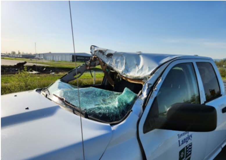
Figure 3. Pickup truck damaged by the occurrence aircraft (Source: TSB)
