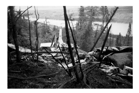
damage to the wings, the seaplane had a left roll attitude of 15 to 20 degrees, was nose-down, and on a heading of 113 degrees magnetic when it struck the ground. The damage attributable to the impact and the nose-down attitude of the wreck are consistent with a loss of control following a stall.
