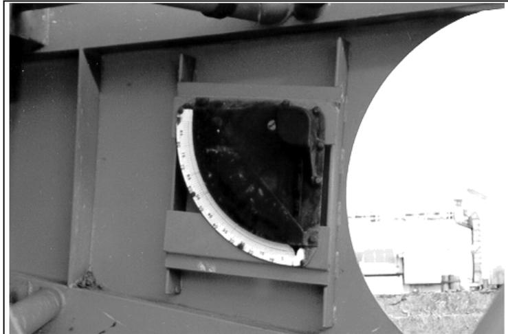
Although an inclinometer was attached to the boom and visible from both the operator's position and from the barge's deck, neither the operator nor his supervisor considered the angle of inclination when the crane was being prepared for the transfer.
