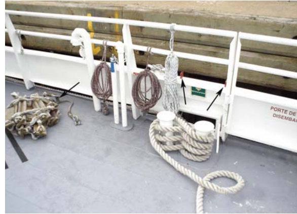
Photo 6. Port side Jacob's ladder secured to the main deck (left-hand arrow) and points for attachment when deployed (right-hand arrows)
