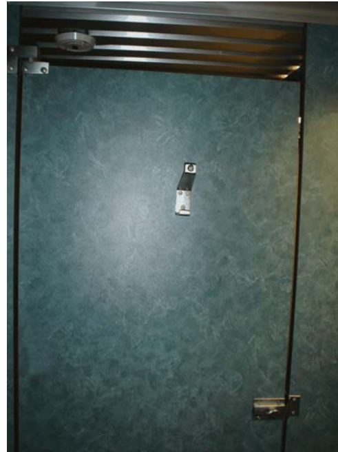
Photo 3. Aft-facing steel coat hook on the inside of the washroom door
