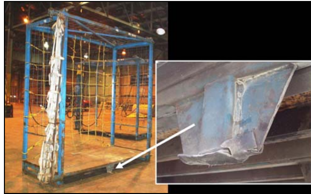
Photo 3. Metal cage with support feet deformed by the explosion
