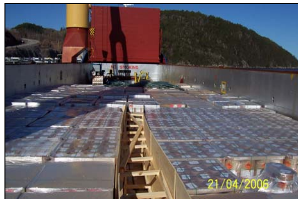
Photo 5. Dunnage between pallets from Sweden
