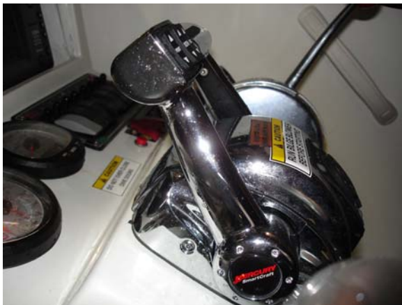
Photo 7. Throttle position (after capsizing) at three-quarters ahead
