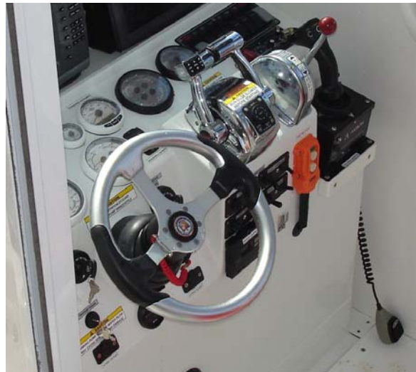
Photo 6. Kill switch and throttle position (note lanyard draped over steering wheel)
