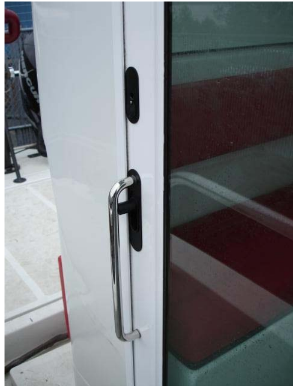
Photo 3. Looking aft at the starboard door handle and latch (installed upside down)
