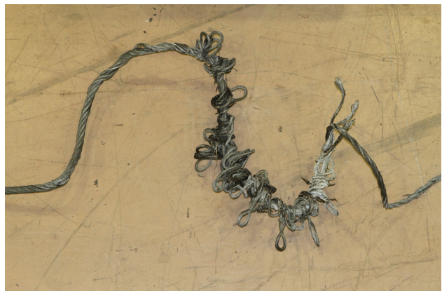
Photo 5. Section of west cable showing "bird cage" and the reduction of the cable from 6 strands and core, down to 3 strands
