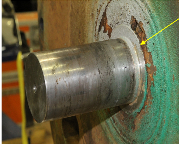
Photo 3. The outboard end of the east idler wheel axle; note the stepped section (arrow)
