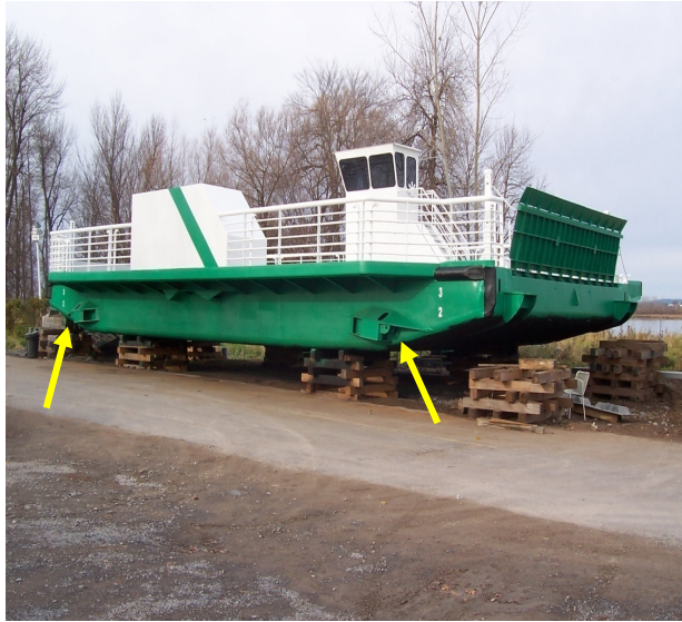
Photo 8. The Ecolos showing the location of the west cable roller fairleads (arrows)
