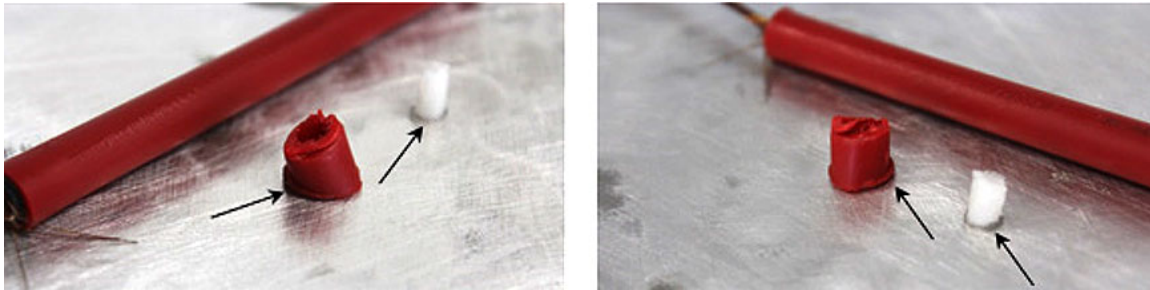
Figure 4. Polythene fragments starting to melt at the surface of the plate (indicated by arrows) at 113 °C
