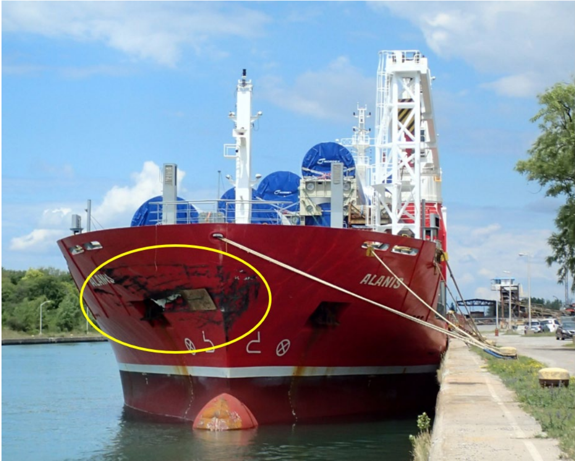
Figure 10. Damage to the forward starboard section of the Alanis's hull (circled) (Source: TSB)
