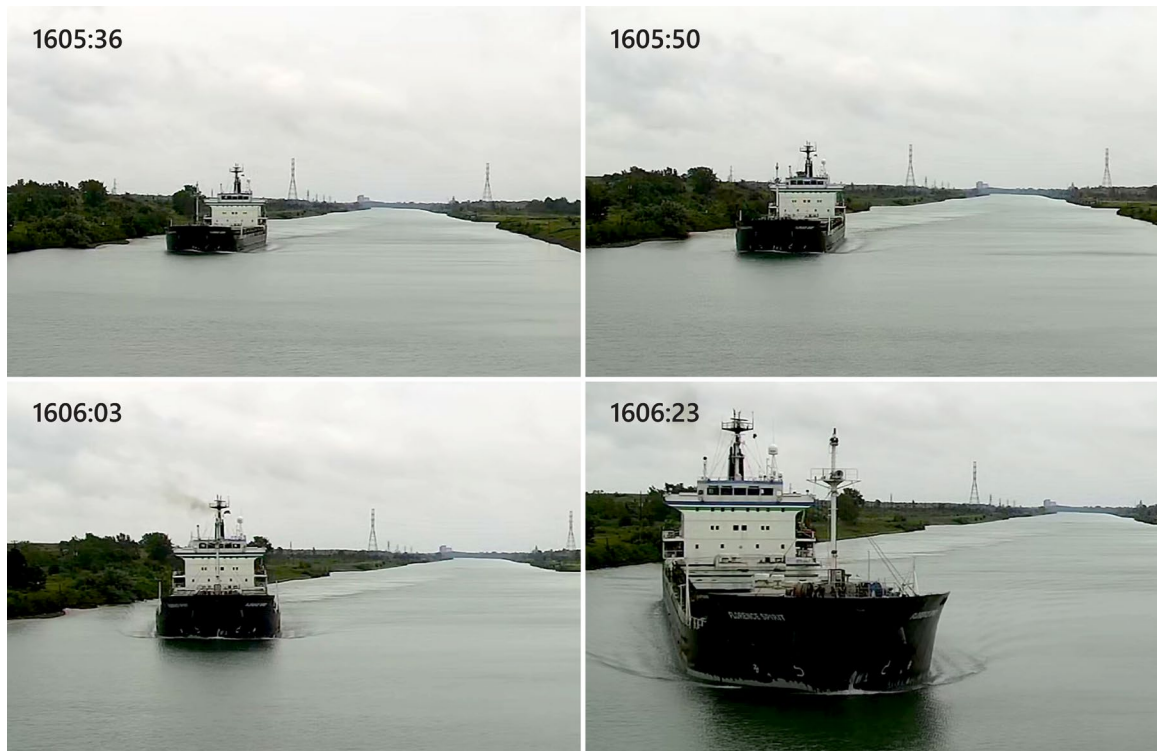
Figure 7. Four images taken prior to the collision, showing the Florence Spirit sheering to port over a period of 47 seconds, as seen from the Alanis (Source: ALANIS / Rambow Bereederungs GmbH & Co. KG)
