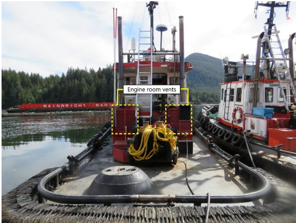
Figure 2. View of the Ingenika from aft, showing engine room exhaust vents (Source: Third party with TSB annotations)
