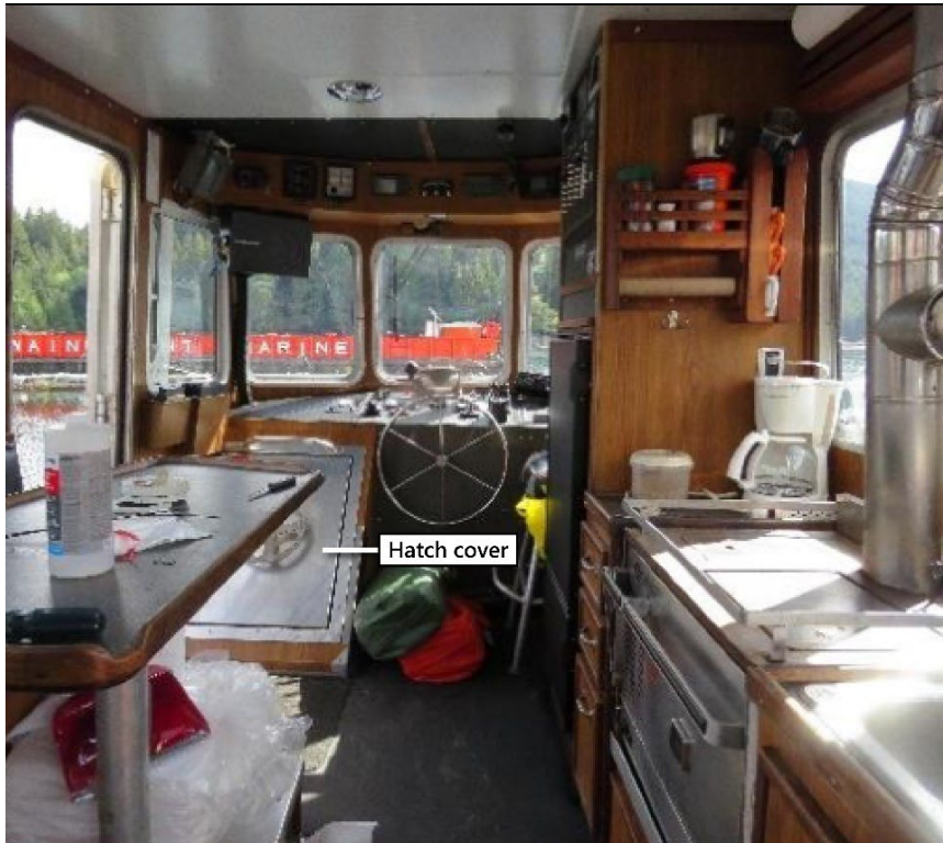
Figure 5. View of wheelhouse showing hatch leading to the accommodation (Source: Third party, with TSB annotations)
