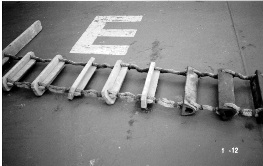
LOWER SECTION OF PILOT LADDER WITH THREE BOTTOM STEPS OF HARD RUBBER OF COMPARABLE STRENGTH OF HARDWOOD. NOTE STEPS AT VARIOUS ANGLES DUE TO SLACK CRIMPING. THE LOWEST BATTEN IS AT THE NINTH STEP INSTEAD OF FIFTH.
