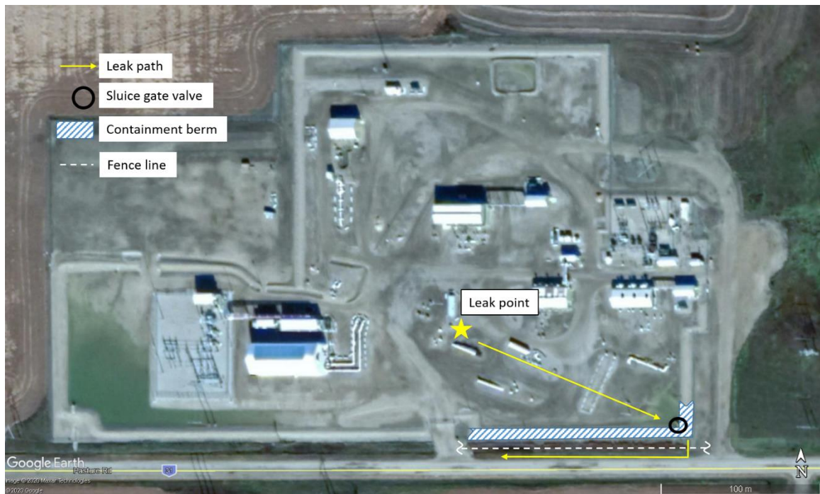
Figure 6. Overview of Herschel pump station indicating the release path (Source: Google Earth, with TSB annotations)
