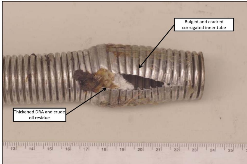
Figure 5. Failed corrugated inner tube of the ¾-inch flexible braided hose (braid removed), showing thickened DRA and crude oil residue (Source: Enbridge, with TSB annotations)
