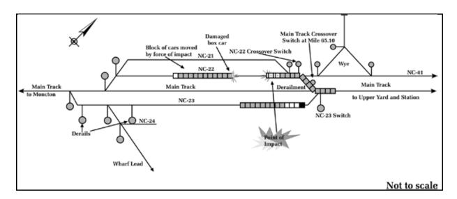
The locomotive engineer at the controls could not recall exactly what led him to believe that the main track crossover was lined in the reverse position—the switch target, the switch points, or both. The emergency brake was applied. Realizing that the train was going to be diverted into track NC-22 and collide with standing cars on that track, the crew members threw themselves to the floor and braced for impact.
