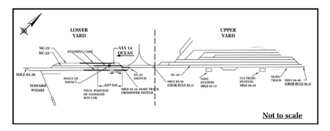
The yard tracks in Miramichi extended from Mile 66.4 to Mile 63.5. There were two separate yards, known as the upper and lower yards (see Figure 3). The two yards were joined together by the main track and by track NC-41 which, when it reached the main track crossover at Mile 65.1, was redesignated track NC-22 in the lower yard. The main track was tangent from Mile 66.4 to Mile 64.0. The track grade was minus 0.8 per cent descending for eastward trains.
