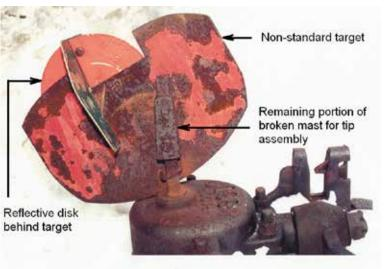
rusted, including the fracture surfaces. It was equipped with four bolt holes to permit the fastening of the tip targets directly to it by nuts and bolts.
