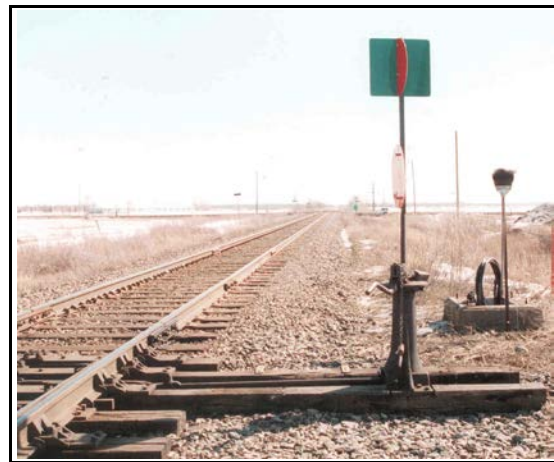
Figure 17 - Top photographs show switch points open 3/16 inch yet a green CTC signal is displayed to a train crew. Bottom photographs show an unlocked and partially raised switch handle, yet a green switch target.
