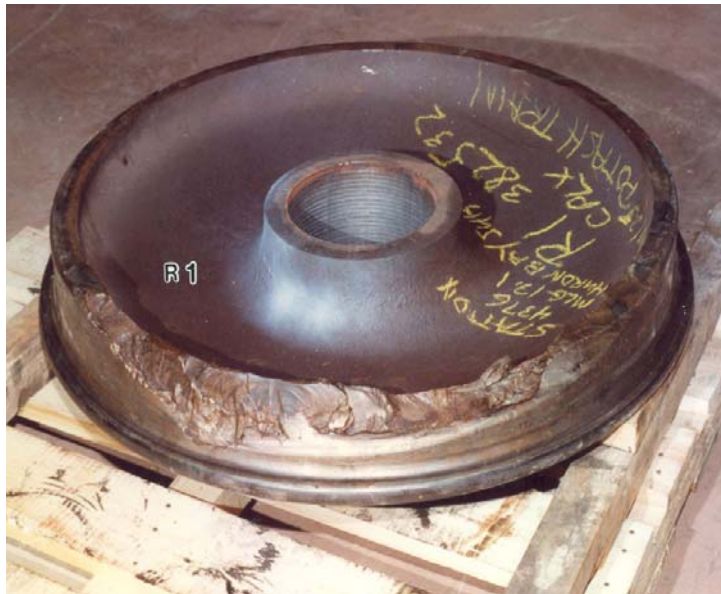
Photo 3. Broken R1 wheel from car CPLX 382532
