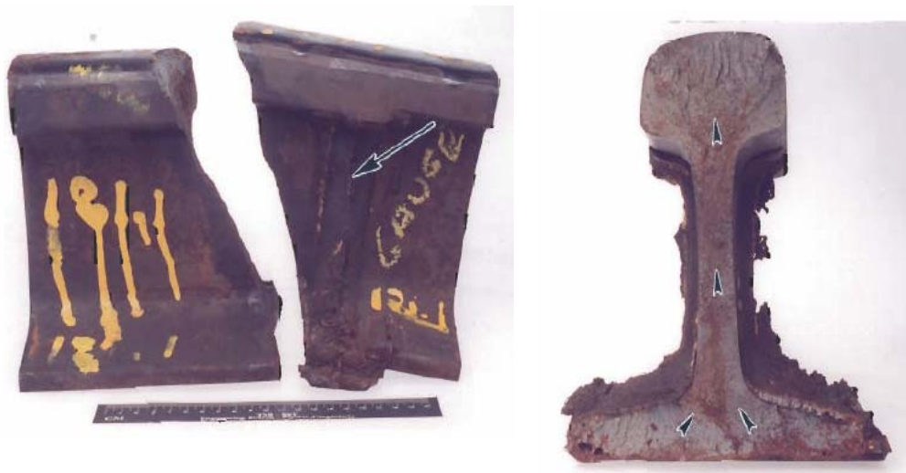
Photo 1. Broken rail from Mile 121.10. The arrow on the left image shows the location of the thermite weld. The arrows in the right image show the direction of the chevron fracture pattern.
