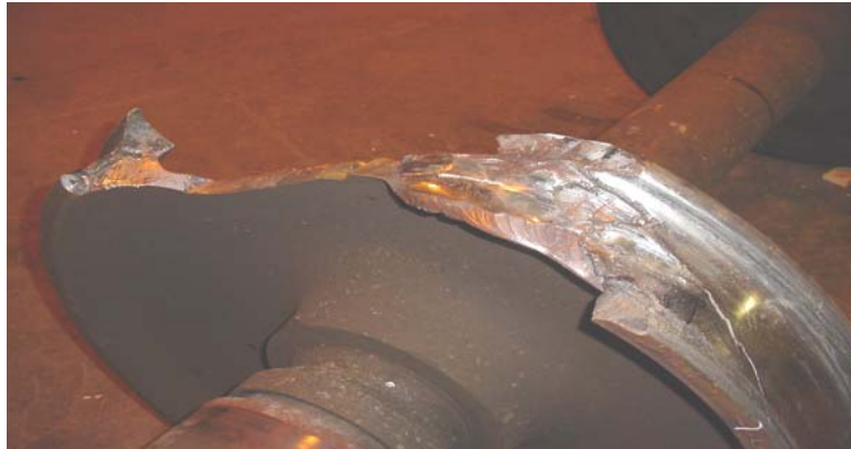
Photo 4. Broken wheel from car CNWX 111231
