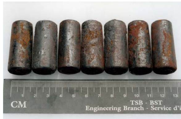
Photo 3. Inner rollers from R-2 bearing
