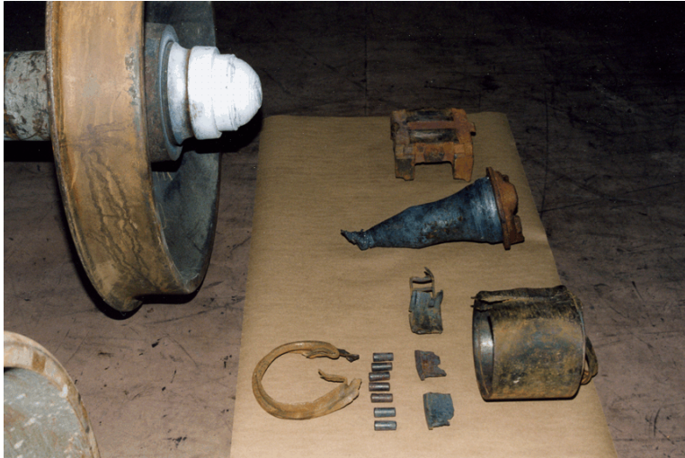
Photo 1. Wheel and axle journal (R-2) with some of the recovered pieces
