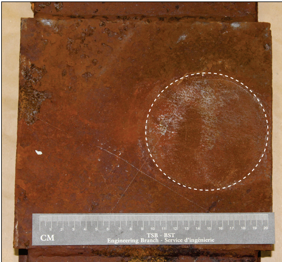
Photo 5. Coupler pin carrier plate showing eccentricity of wear marks
