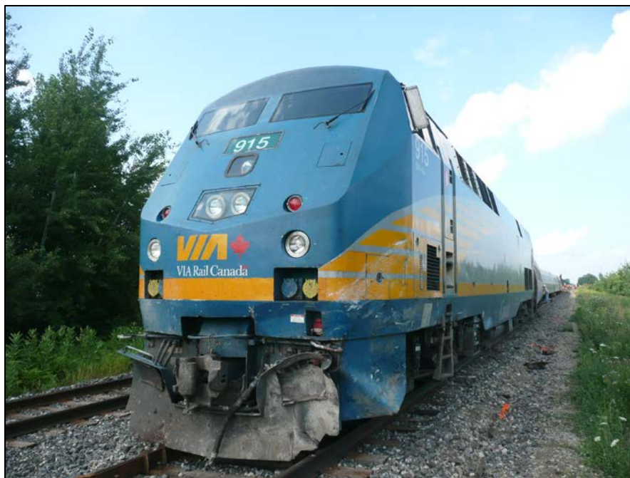
Photo 1. VIA 71 locomotive with damaged pilot
