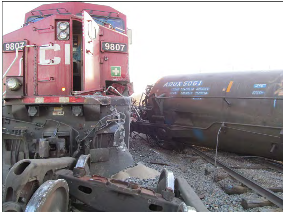
Photo 3. Damaged stationary locomotive and jackknifed AOUX 5061
