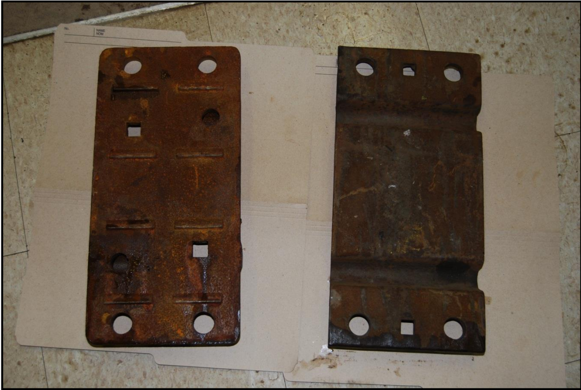
Photo 7. Bottom of plates (Note: lugs on bottom of cast plate [left] and smooth bottom of rolled plate [right])
