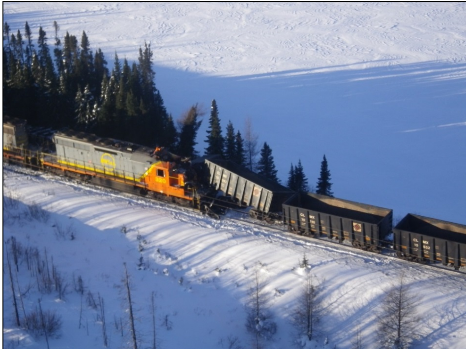
Photo 1. Train FCN-05 in collision with the tail end of train BNL-005 (source: QNS&L)
