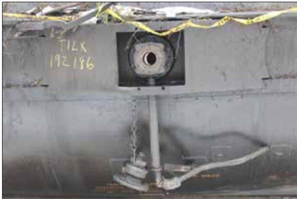
Photo 7. Car TILX 192186 BOV and bent handle
