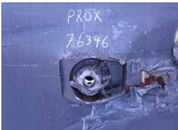
Photo 11. Partially open BOV of car PROX 76346
