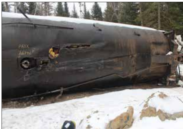
Photo 10. Car PROX 76346 jacket damage
