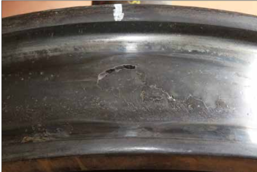
Photo 12. Shell on L1 mate wheel tread contained within non-condemnable slid flat
