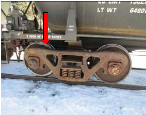
Photo 2. Broken R1 wheel (source: CP Police)
